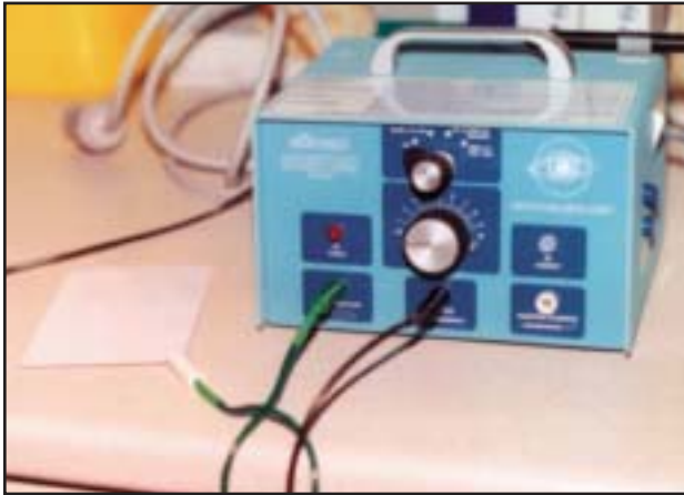
Figure 2. Electrosurgery unit, Ellman Surgitron.
